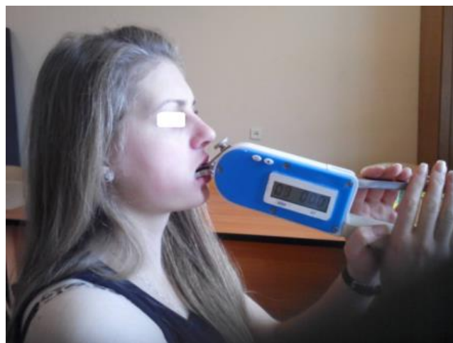
Fig. 2. Active dosed mechanical therapy – after feeling pain patient consciously grips jaw (hear audio signal) which lead plate of the device to its primary position – mouth closed
