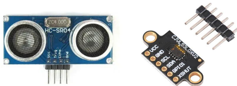
Fig. 2. Sensors used to build the information system network: a) ultrasonic HC-SR04, b) infrared VL53L0X
